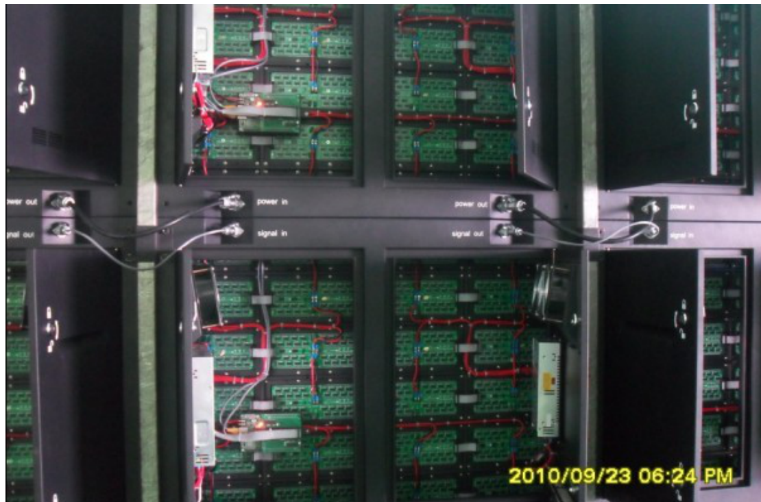
Signal and Power Cable, and Iron Tighten Plate Connection Between Cabinets.
