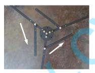
5. Swing the stabilizer arms, counter-clockwise until the end hole lines up with the bolt from the other legs. The legs may need to be pushed or pulled to align the holes and bolts.
