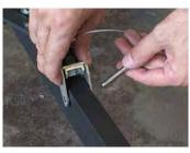
9. Swing the turnbuckles down to meet with the legs of the dolly. Use the pins to attach the turnbuckles to the legs. NOTE: You may need to turn the turnbuckle to get the holes to align.
