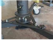
7. Remove the knob and bolts from the base of the column. Then set the column onto the dolly center plate so that the holes align.
