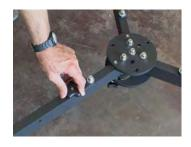
4. Remove the 3 knobs holding the stabilizer arms in their folded position.
