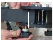
2. Pull the knobs under the dolly center plate to release the legs from their stored position and swing the legs out into working position.
