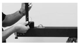
Pull the pin out from the cable guide baseblock. Lift the cable guide and insert the pin to secure.
