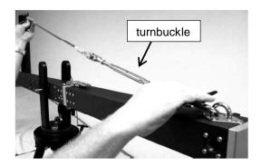
Next, place the cable over the cable guide and secure the other end to the latch point at the front of extension section 1.
