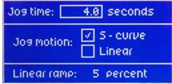
Under the "jog time" option, you can set the number of seconds the Head will take to go from mark to mark, from zero to mark, or from mark to zero.
