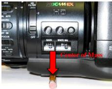
With smaller cameras (under 10lbs), you may not need to adjust the vertical balance. For larger cameras, you may want to adjust it for optimal performance and to minimize the effort the servos have to make to hold position. To get the vertical balance right, raise or lower the platform to get the camera's vertical center of mass located on the center of tilt
