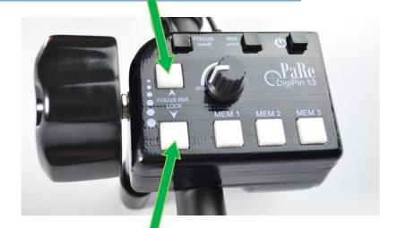
Also, when focusing closer we can set the lower limit by briefly pressing the focus lock button.
