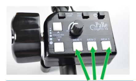
When you want store of current focus value, pres and hold MEM button (1, 2, or 3) while the neighboring button start blinking what is sign that current value is stored on that MEM button.
