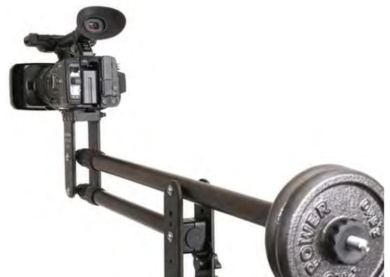
If you keep your hands on the jib, you may be able to operate it without the tilt or pan brakes tightened. If you need to take your hands off the jib, you may want to tighten the tilt and/or pan brakes to hold position. These brakes are not hard-stop mechanisms, they are soft-stops that can be pushed-through.
