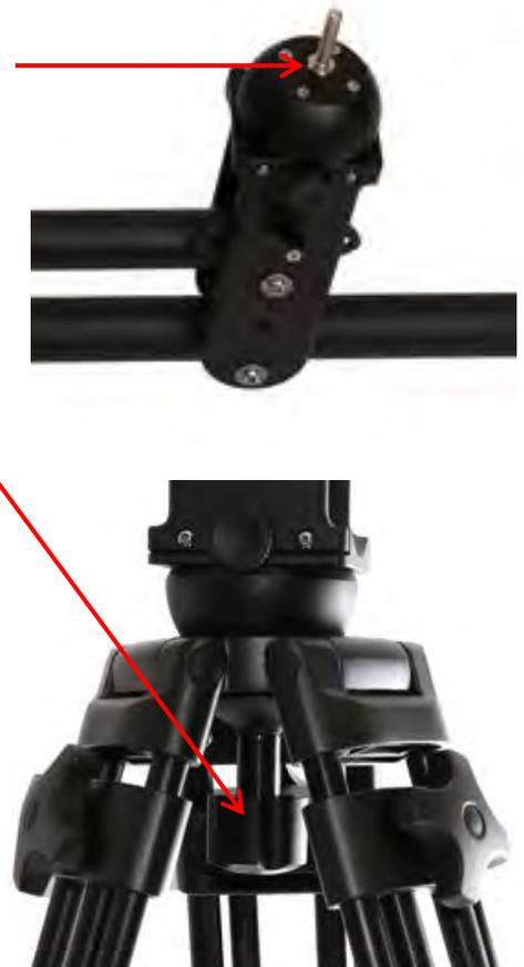
**Option B (flat-base tripod with 3/8"-16 stud)** - If you're mounting to a flat-base tripod with 3/8"-16 stud, the jib base will thread directly onto that stud. Use the set screws on the flat base to prevent loosening.
