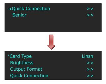
(6) After setting, turn the rotary knob, select <Quick Connection>, push the rotary knob to confirm for next setting, shown as follows:
