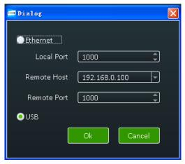
Finally, select Ethernet or USB connect, click "Ok", and finish connecting. The green square in the bottom right means the connection is successful, white red is not.
