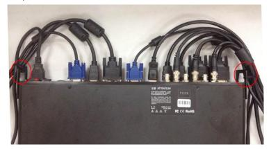
For connector protection and for additional cable support this product is fitted with protection frames on either side of the device. For cable support use cable ties to attached to the protection frames to avoid stress on signal connectors.
