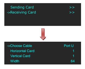
(8) Set the horizontal card, vertical card, width and height. For example, set horizontal card as 3, vertical card as 2, width and height as 120, shown as follows:
