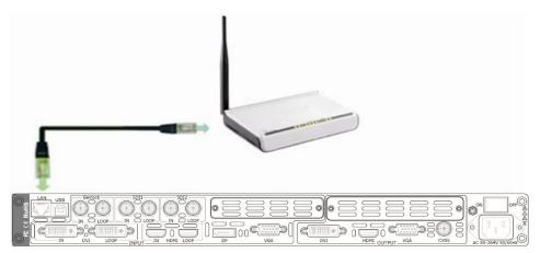
The second step: IP address setup. Please refer to IP Setup steps which in the "Connecting to an Ethernet Network" section. (Make sure that processors IP address and router IP address are in the same band.)
