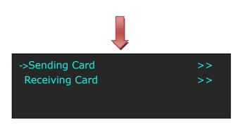
(7) Turn the rotary knob, select <Receiving Card>, push the rotary knob to confirm. Turn the rotary knob again, and select <Choose Cable>, push the rotary knob to confirm. Turn the rotary knob, select Port U and push the rotary knob to confirm.
