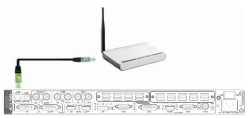
Step two: IP address setting (processor's default IP address is 192.168.0.100)
