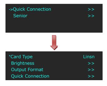
c. After setting, turn the rotary knob, select <Quick Connection>, push the rotary knob to confirm for next setting, shown as follows:
