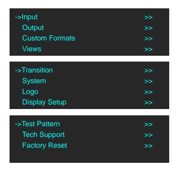
There are 11 menu items in the main menu, and display in 3 pages. Turn the rotary knob, and select any menu above, push the rotary knob to confirm, the OLED display will show the submenu. If push the MENU button, the OLED display will return to the last level menu.
