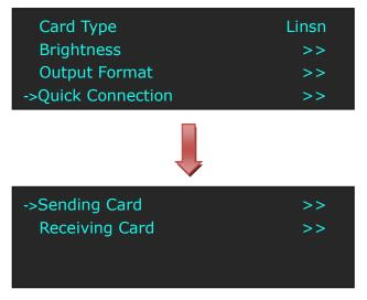
d. Turn the rotary knob, select <Receiving Card>, push the rotary knob to confirm. Turn the rotary knob again, and select <Choose Cable>, push the rotary knob to confirm. Turn the rotary knob, select Port D and push the rotary knob to confirm.
