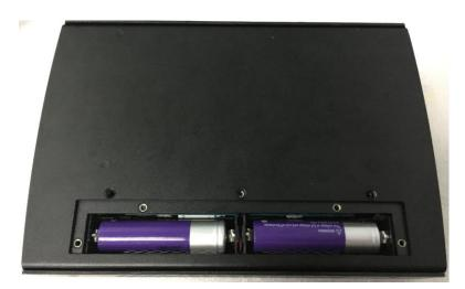
4. Install the holder, and lock the 7 screws, installing batteries is finished. As shown in the figure below:
