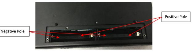
3. Install the 2 lithium ion batteries to the battery compartment one by one. Install the negative pole first, if install the positive pole first, maybe the battery can not be installed, or the battery compartment may be damaged. As shown in the figure below:
