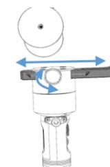
6. Last adjustment is the Yaw axis. Hold the stabilizer sideways and observe the roll motor. Adjust the yaw arm in and out till the roll motor no longer rises or falls.
