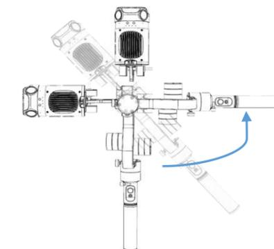
Tilt the gimbal by 45 degrees, the gimbal will automatically orientate to the horizon. Rotate your arm so your elbow points outward from your body. Your hand and gimbal will now be horizontal. Note if the gimbal comes in contact with itself it will destabilize and need to be restarted.
