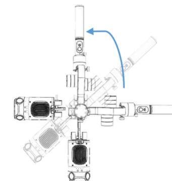
Continuing on from the horizon orientation. Tilt the gimbal another 45 degrees to invert the stabilizer. Rotate your arm so your elbow points upwards. Your hand and gimbal will now be inverted. Reverse or continue this process to return the stabilizer to default orientation.
