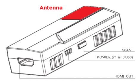
Antenna Area keep free and in 60 degree direction to transmitter for best performance !
