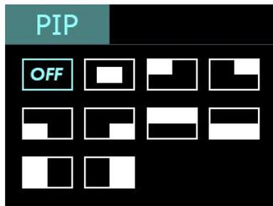
Push SW button 3 times to open PIP menu. PIP menu offers 9 layouts for main picture and sub picture.
