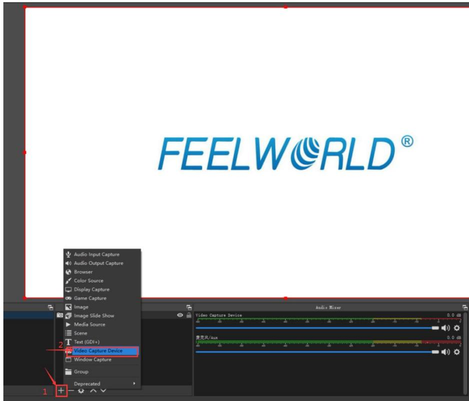
💡 If there is no video format YUY 2 after setting above, check the USB 3.0port connection. Make sure it is linked to USB 3.0port on PC by USB 3.0 cable. (USB 3.0 cable or port is standard in blue while USB 2.0 is in black)
