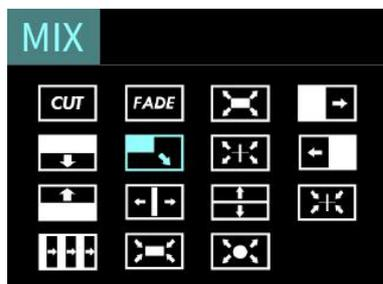
Push button SW to open up the transition effect menu. Use knob to select the desired transition effect icon and push the knob to confirm.
