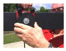
25. Install the sliding counter balancing weight on to the Tail Beam. Slide it up or down the beam to micro balance the EZ Crane.
