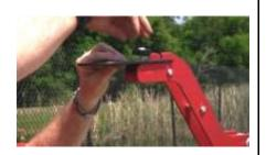
13. Attach the camera mounting plate to the goose neck. Slide the plate and align the notches to center the hole. Secure it with the provided knob.
