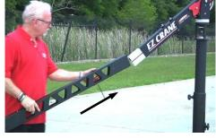
Find the Crane Beams in the bag and build the Crane in sections.
