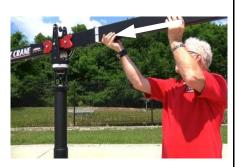
Find the Tail Beam and attach it to the opposite end of the Crane. NOTE: The Tail Beam has double expansion set screws so be sure to expand all 4 set screws.
