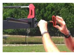
24. Insert the counter weight bar into the mounting hole on the tail arm. Use the hex tool to push the internal set screw and secure the bar in place.
