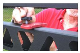
18. Attach cable hitches to the Crane Beams.
