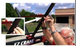
Connect both sides of the red VPole Cross Bar to the cable poles using the included knobs.
