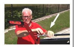
14. Level the camera plate by expanding or contracting the turnbuckle at the end of the parallel beam.
