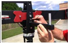
30. Add the Monitor mount bracket to the center post of the Crane. You have the option of placing it on the right or left side of the Crane, depending on your preference.
