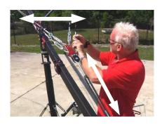
28. Align the suspension of the Crane using the turnbuckle system. The large master turnbuckle will pull all cables simultaneously while the smaller turnbuckles give you control over left/right alignment. You may need to tweak the alignment later after the camera is added but it is easier to this before hand.
