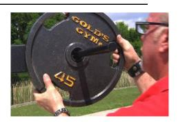
27. Add the counterweights needed to pre- balance the Crane.
