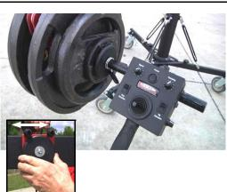
32. Add additional counterweights to compensate for the camera weight. Remember to include joysticks and zoom controls as part of the counter balancing. Micro balance with the sliding counterweight.
