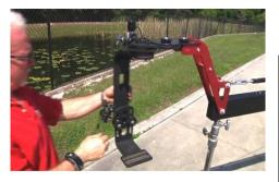
29. Mount your remote pan/tilt head and camera to the end of the Crane. Use the mounting knob provide in the tool bag.
