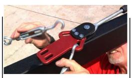
Attach the turnbuckle ends to the wide (outside) hitches on the turnbuckle bracket.
