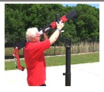
Set the Center Beam onto the Pedestal or support system and secure it down with the washer and knob.
