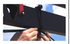
31. Attach the cables for pan, tilt, zoom, focus, monitoring, etc. and dress them on to the underside of the Crane using the bungee ball tie downs provided in the canvas tool bag.
