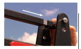
10. Attach the Parallel Beams. Start with the short beam. Insert the male end into the female connector at the Center of the Crane. Use the hex tool to tighten the internal set screw unit the tip protrudes through the capture hole on the underside.
