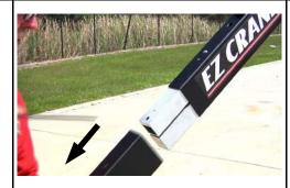
5. Use the Hex tool provided to loosen the expansion set screws and remove the Camera End Beam. Set it aside to be attached to the end of the Crane later.
