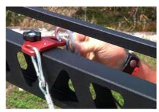
Starting with the longest cable (red) cables, clip the carabineer ends to the cable hitches.
