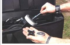
Find the mounting hardware (shaft, knob and washer) in the canvas tool bag. Screw the short end of the shaft into the swivel base of the EZ Crane.
