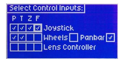
Here is where you can assign how Pan, Tilt, Zoom, and Focus will be controlled.
