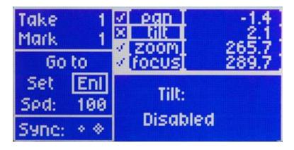
The cursor box then appears in the top right corner, and lets you select one of the four axes. Move the cursor over which axis you wish to control.
