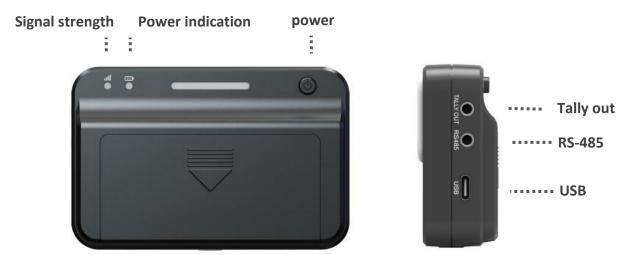
Note: Signal strength indication: when the signal is strong the signal indicator shows green, when the signal is moderate the indicator shows yellow, and when the signal is weak the indicator shows red.
